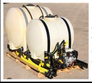
Used part of one season. GX160 Honda recoil start engine with direct coupled centrifugal pump. Agitation in both tanks. Valving manifold to switch between tanks. Unit designed to fit in an 8' pickup box. Does not include hose reel.
