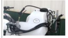
Equipped with 4.9 gpm pump, control switch, 15' of hose, Black Jewel handgun, two Boominator tips producing a 30' swath (15' right/15' left), and on/off right/left control valves
